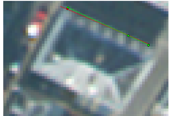
Figure 6: Adjustment results. Extracted points before adjustment (red), after adjustment (green). Segment RMS decreases from 0.37 to 0.27 m.
