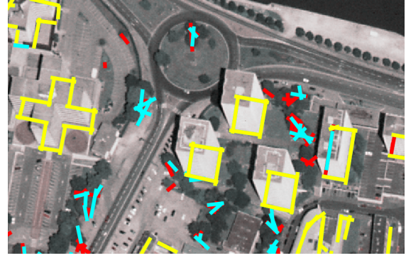
Figure 3: Vegetation filtering. Red segments are discarded using orientation criterion (RANSAC procedure), blue segments with planar criterion. Yellow segments are can be diagnosed.
