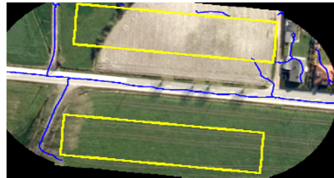
Figure 1: 2D line extraction result (blue) and region mask (yellow) for computing entropy E
