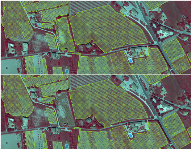
Figure 7: First data set : results of the approaches “frequency analysis” (top) and “classification” (bottom) using per region ML classification algorithm applied to SIFT based texture indexes
