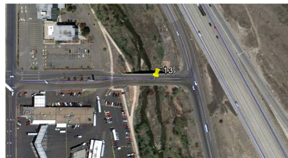
Figure 2. Example of point-to-line matching (Denver, Colorado): only one vector has a matched road name.
