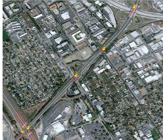
Figure 8 Example of feature coding results (Santa Clara County, California): Blue lines – TIGER road vectors; Yellow markers – NBI records; Red lines (along the blue lines) – feature coded bridge vectors.
