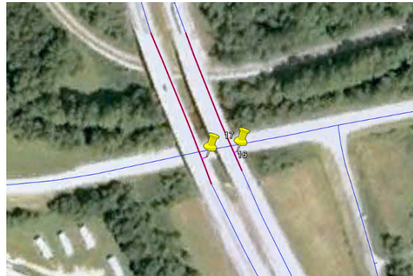
Figure 5 Example of point-to-line matching (Braxton County, West Virginia): two bridges matched with two road vectors, both bridge locations are to the southern ends of the true bridges. The final bridge vectors are shown as red lines.
