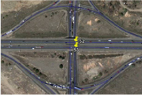
Figure 3. Example of point-to-line matching (Denver, Colorado): two bridges matched with two road vectors, travelling direction has to be used because both vectors have a successfully matched road name.
