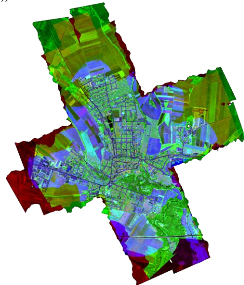
Figure 7. Active multi-wavelength reflectance image estimated from radiometrically calibrated ALS data sets; 532nm (linear scale from 0 (black) to 0.15 (blue)); 1064nm (linear scale from 0 (black) to 1 (green)) and 1550nm (linear scale from 0 (black) to 1 (red)).
