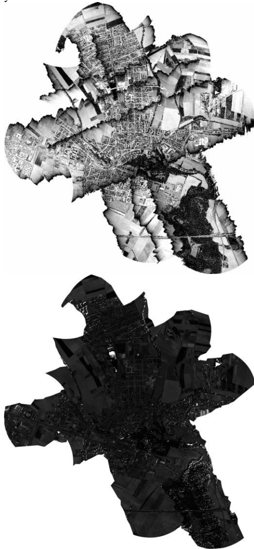
Figure 2. Upper image: amplitude image of the 532nm ALS data of the study area (linear scale from 0 (black) to 1000 (white)); Lower image: Calibrated radiometric reflectance at 532nm (linear scale from 0 (black) to 1 (white)).
