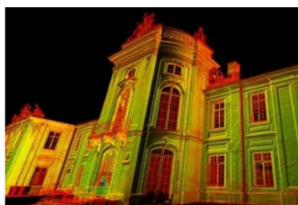
Figure 2. 3D point cloud data produced by laser scanner (Source: http://www.3deling.com/category/3d-laser-scanning/ )
