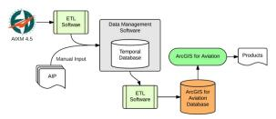
Figure 6. Data flow between data management software and GIS software
