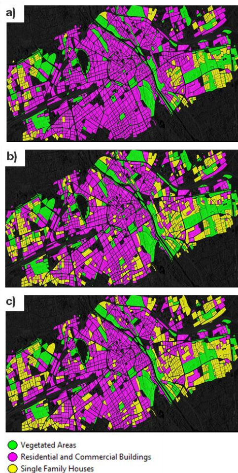
Figure 5. Ground-truth UST map (a), classification obtained with the ensemble of classifiers (b) and the reclassification obtained by the application of the CRFs model (c).
