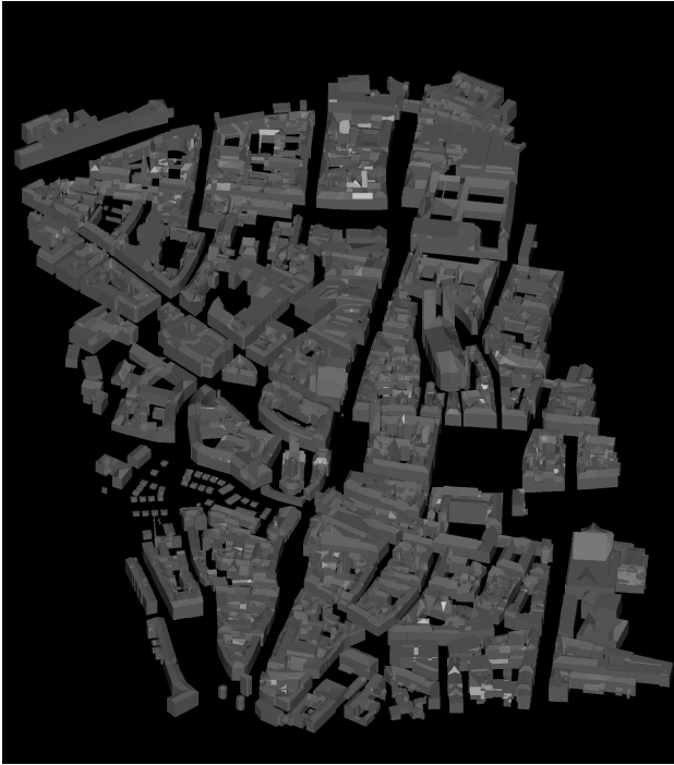
Figure 7. Rendered image of CityGML model, representing the line-of-sight of the virtual SAR sensor.
