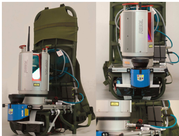
Figure 2. Images of the backpack system. Left: Side view with all of its sensors and equipment. Right: Detailed view of the SICK and the switch.
