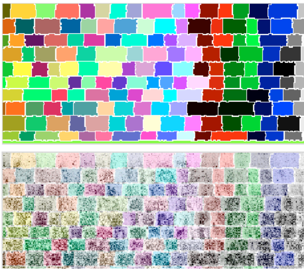
Figure 6 Segmentation of an intensity image created from MLS data: watershed segmentation results (top); superimposition of segmented image and original image (bottom).
