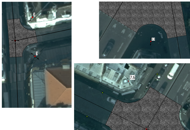
Figure 4: 3 different radius size (3m, 4.9m, 7.6 m) for streets of various importance, from real Paris data
