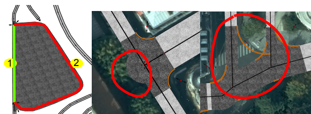
Figure 14: Various cases of failure from more severe to less severe (1, 2, 3). 1 : loop, 2 : bad buffer use, 3 : radius too big for network.
