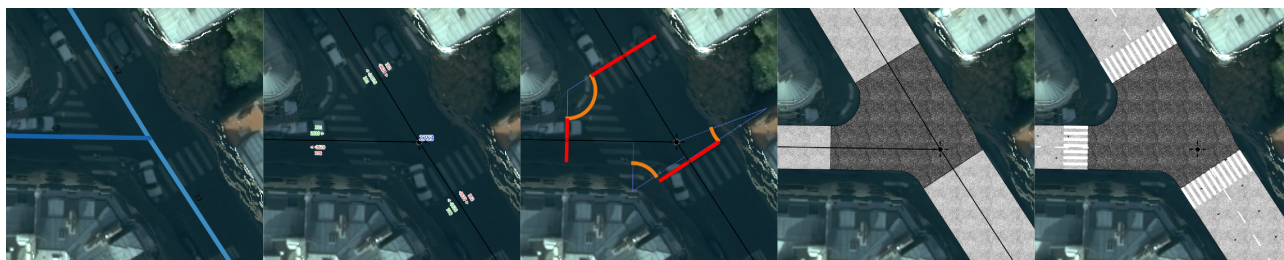
Figure 1: StreetGen in a glance. Given road axes, reconstruct network, find corner arcs, compute surfaces, add lanes and markings.
