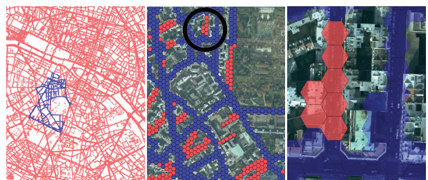
Figure 8: Visualisation of to-do hexagonal map. Blue when sensing data, red otherwise
