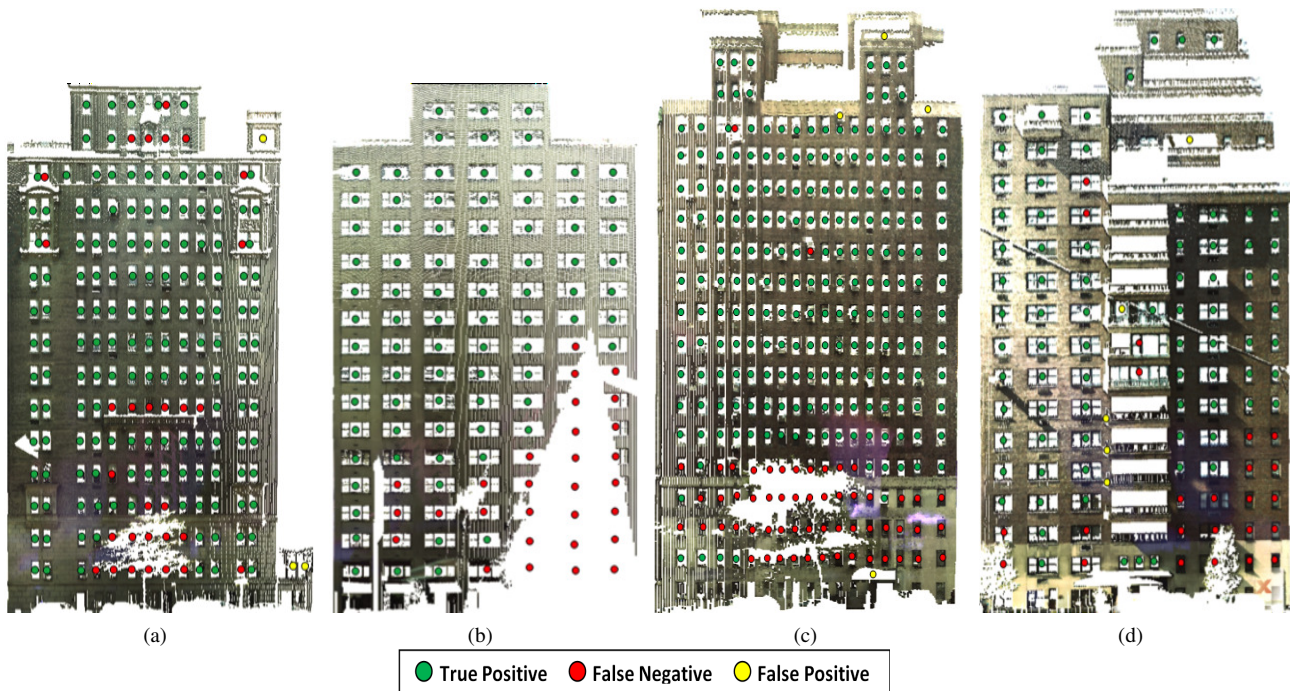
Figure 5: Window detection results are shown for some façades. In (a), (b) & (c) we can see a number of false negatives due to occlusions. In (c) & (d) we also find some false negatives due to closed windows because of window shutters or curtains.
