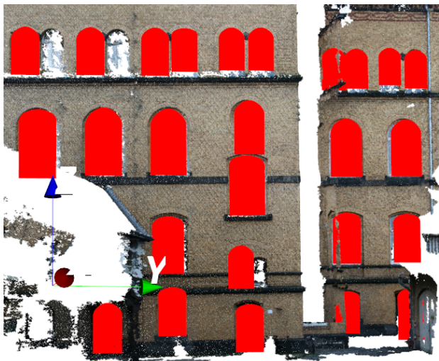
Figure 10: Two top left windows are not localized. This is because these windows are too close the neighbouring windows and their hypothesis overlaps these neighbouring windows and gets vote out due to the overlap. In general, we can remedy such problems by allowing many more samples that would increase the probability of getting a global maximum, i.e., in this case getting exactly two non-overlapping but very close windows.
