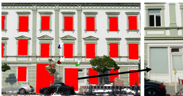
Figure 11: The left facade shows localized windows and doors (filled red polygons) of a facade. An image of a part of the facade is depicted on the right. The arrows shows a false localization of a door.
