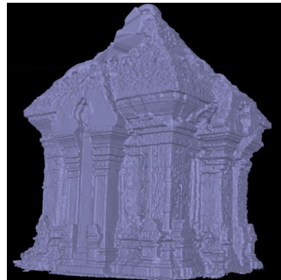
Figure 16. Po Dam Tower, the achieved 3D mesh by Photoscan Agisoft (SfM)
