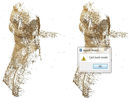
Figure 10 The problems during the alignment process using images acquired with a non correct set up of the equipment.
