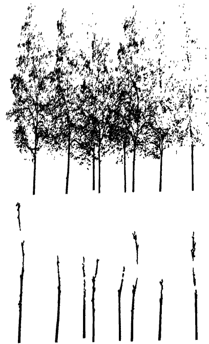
Figure 8. Results of tree stem detection: Original data set (upper) and detected tree stems (lower)
