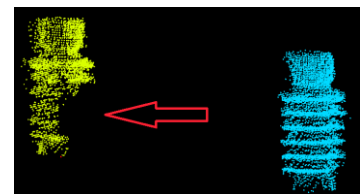
Figure 12. An occluded insulator which is not detected shown by a red arrow
