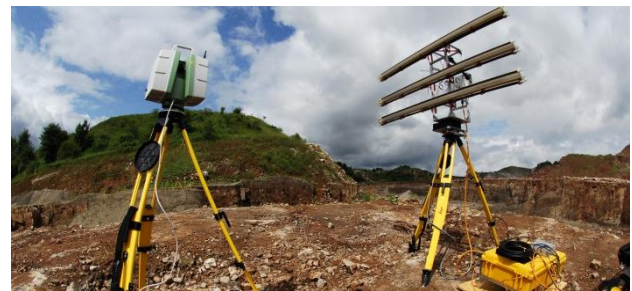
Figure 1: Leica C10 TLS (left) and GAMMA RADAR scanner (right)
