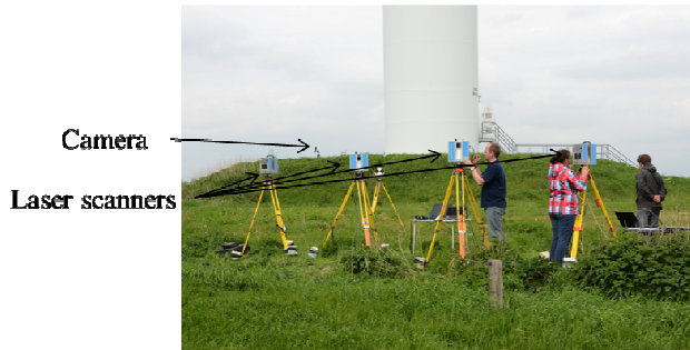
Figure 4. Measuring arrangement of the camera and laser scanners
