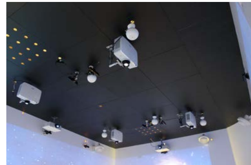
Figure 2. An image of projectors, kinects and fans are installed on the ceiling.
