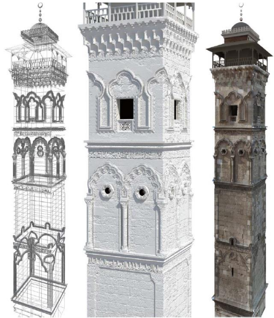
Figure 34 – Wire-frame, solid model and render (by W.Wahbeh and A.Aboufares)
