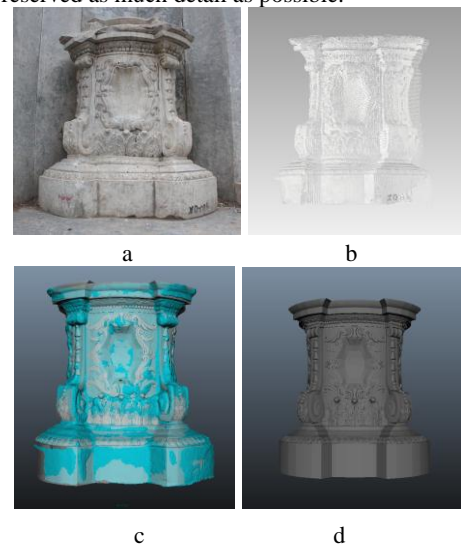
Figure 12. a. Element at site; b. Point Cloud data; c. Generating low poly model from high res model using topology technology; d. Low poly model
