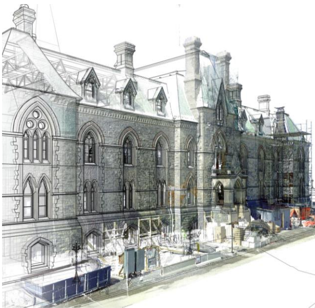
Figure 12. Results of the East Façade (LoD 3) of the BIM with point cloud overlay.
