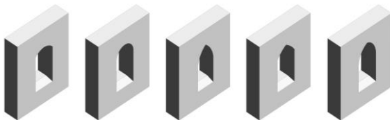
Figure 3. Various examples of round-headed and pointed arch configurations producible with the single parametric opening model.
