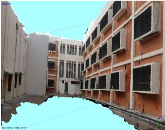
Figure 15: Textured 3D model of one portion of building at civil engineering department
