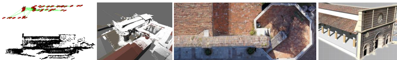
Fig. 1. Some phases of the true-orthorectification process with the UAV images acquired over the Basilica di Santa Maria di Collemaggio. From left to right: image orientation, dense model generation, true-orthophoto mapping and 3D projection on a BIM.
