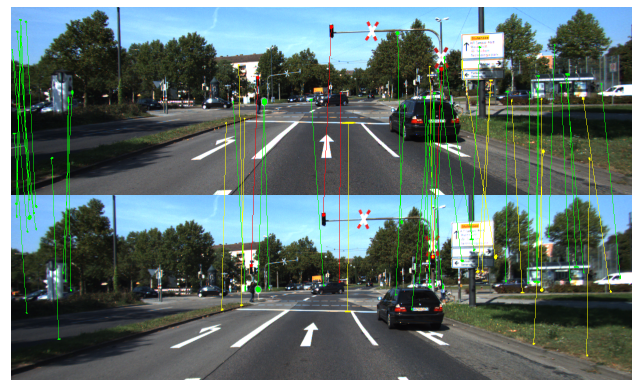
Figure 7: The red, yellow and green ellipses are matched in left and right images.
