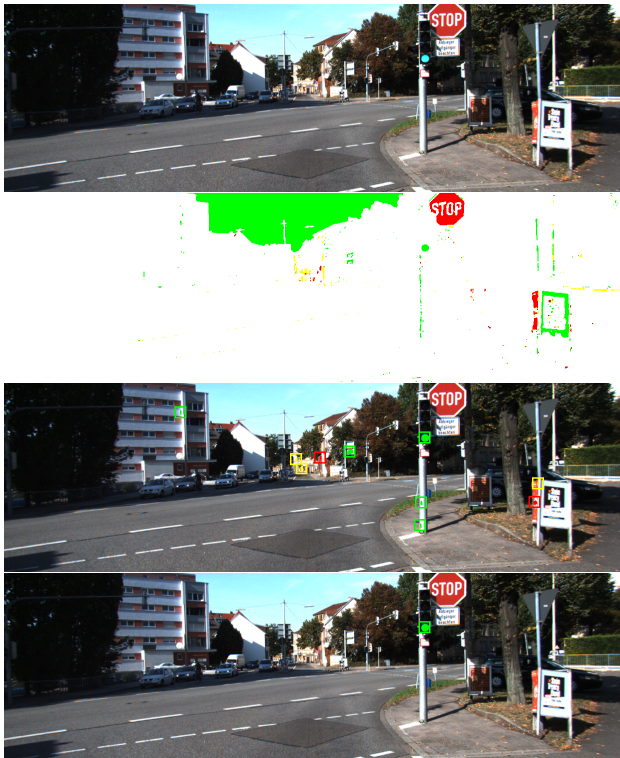
Figure 9: The traffic light detection algorithm using mono camera (third row) has a few false positives. The stereo cameras approach (fourth row) does not contain any false positive while it maintains the true positives.
