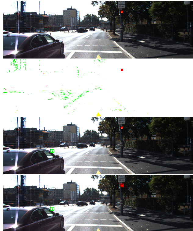
Figure 10: The traffic light detection algorithm using mono camera (third row) can not correctly detect the traffic light and a false positive incorrectly labeled as traffic light. The stereo cameras approach (fourth row) correctly detects the traffic light although a false positive is detected too.
