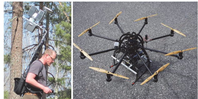
Figure 1. The backpack laser scanner (AkhkaR2) and the UAV-operated laser scanning system.
