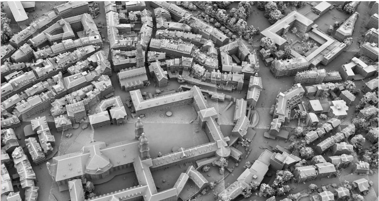
Figure 10: Larger part of the mesh generated from the airborne oblique data set. Visible tile overlaps are due to shading and not to variances in geometry.
