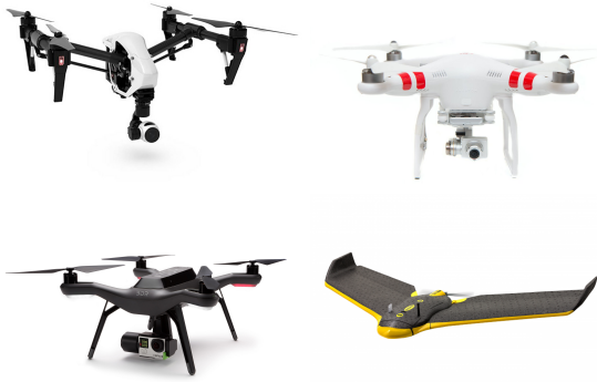
Figure 2: Evaluated drones: DJI Inspire 1 (top-left), DJI Phantom 2 Vision+ (top-right), 3DR Solo with GoPro HERO4 (bottom-left) and senseFly eBee (bottom-right, used as a reference with a global shutter camera).
