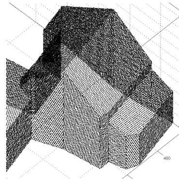
Figure 3: Result of the point sampling for each face of the boundary representation (bird’s eye view) with sampling distance 20 cm and  $\sigma = 3$  cm for each coordinate. The points of the bottom area have been omitted for clarity.
