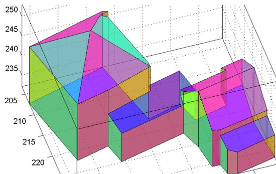
Figure 8: Constrained boundary representation as the result of the reasoning and adjustment process. 38 functionally independent constraints have been recognized and enforced, cf. Table 2. The reasoning process led to a more adequate representation of the pyramidal broach roof.
