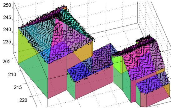
Figure 2: Detail of a point cloud obtained by airborne laser scanning and the derived generic polyhedral building reconstruction.
