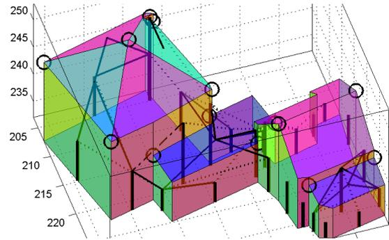
Figure 7: Illustration of all constraints between faces recognized by the hypotheses tests: identity (—), orthogonality (---), parallelism (···), concurrence (○), verticality (vertical poles). Constraints with the bottom area of the building are omitted for clarity.
