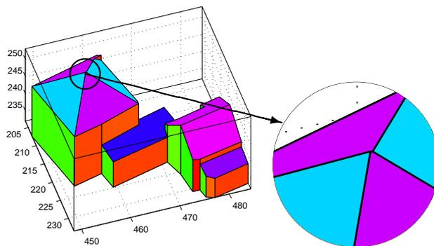
Figure 1: The pyramidal broach roof has been reconstructed as a hipped roof with a very short ridge line. The adjustment process enforces the concurrence constraint and therefore changes the topology of the roof to a pyramidal roof.
