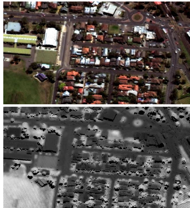
Figure 5. Colourised LiDAR points with colour (top) and NDVI images (bottom) for a small area.
