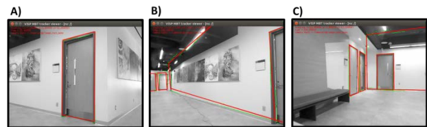
Figure 1. Sample frames demonstrating the ViSP model-based tracker. The second floor of York University's Bergeron Building is being observed, the 3D building model is projected onto the image plane (red lines) using the previous epoch's camera pose, matching is performed and the current camera pose is estimated (Li-Chee-Ming and Armenakis, 2016).
