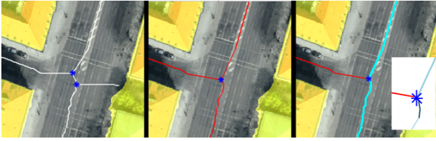
Figure 1: Main steps of chain forming algorithm. Left: vectorization by means of medial axis; forbidden areas are indicated by the golden color. Middle: The implausible segments are filtered out. We also recommend fusing junctions (denoted by blue crosses) in order to increase the number of neighbors for chain forming (right image). Two segments are fused into a chain (cyan), because their partial dominant direction were similar. The red segment is a side road in this case. Chains and side roads are the main input for the chain-wise generalization, see Sec. 4.
