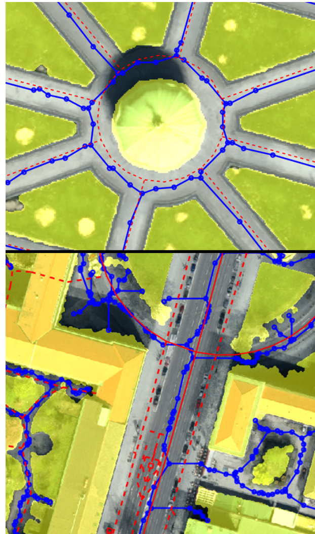
Figure 2: Detailed view of the classification results, where non-road class is emphasized by golden color, the input polylines, in blue, and the “ground truth” represented by the content of the OpenStreetMap shapefile, in red. Here, main and auxiliary roads are depicted by solid and dashed lines, respectively.
