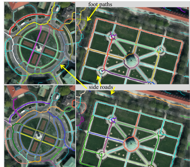
Figure 4: Detailed view of chain forming in case for two traffic roundabouts, using partial dominant directions (top row) and RANSAC (bottom row).
