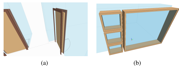
Figure 8: Example of IfcDoors and IfcWindows .
