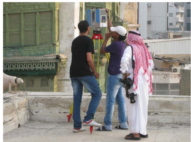
Figure 7. Scanning with Z+F Imager 5006 in Jeddah, Saudi Arabia
