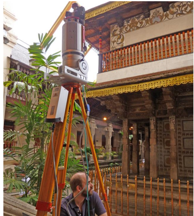
Fig. 3. 3D-Scanning at the shrine with Riegl VZ 400
