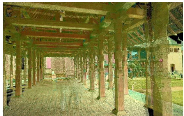
Fig. 4. Point cloud showing the Audience Hall. Combination of reflectance and true colour information
