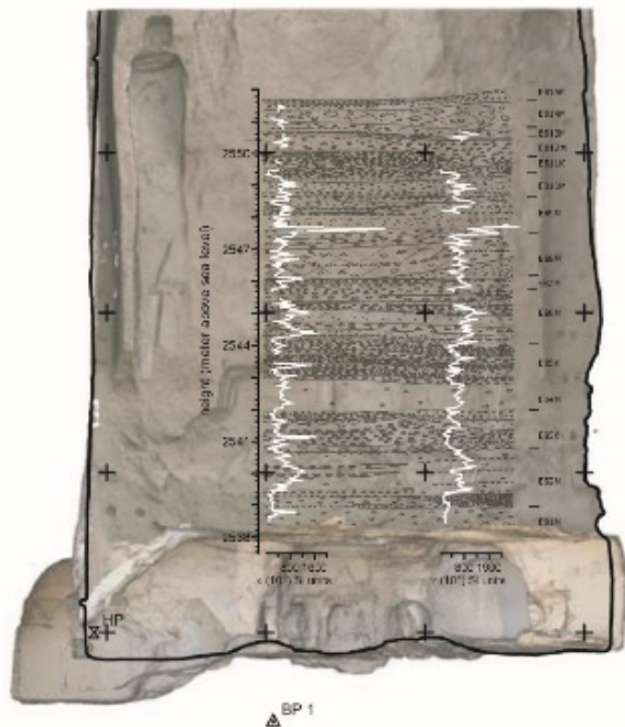
Figure 9. Geological Mapping of the rear side of the 38m Eastern Buddha niche (Urbat 2009)
