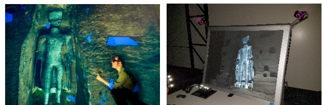
Figure 6. (left): Immersive 3D aixCAVE System 5 (right): infrared head-tracked 3D workbench 5
