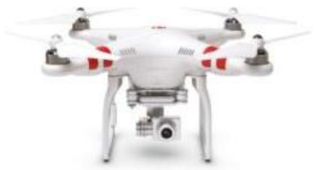
Figure 8. Aerial photogrammetry drone used on site was a Phantom 2 vision +, www.dji.com
