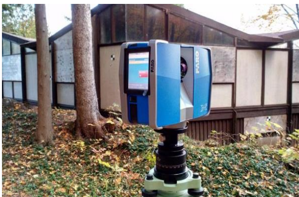
Figure 6. Laser scanning the building with a Faro Laser Scanner Focus3D X330 (above) Photo: Pierre Jouan.
