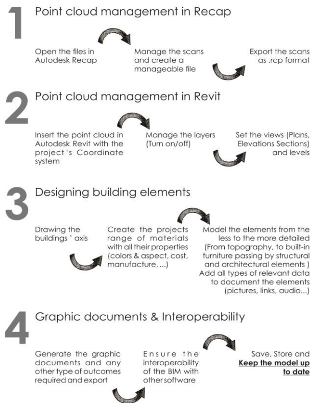
Figure 9. Scheme of the Building Information Modelling (BIM) methodology for the Strutt House, by Pierre Jouan.
