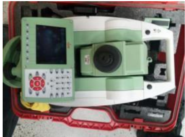
Figure 7. Leica viva TS11, Total Station. Photo: Pierre Jouan.
