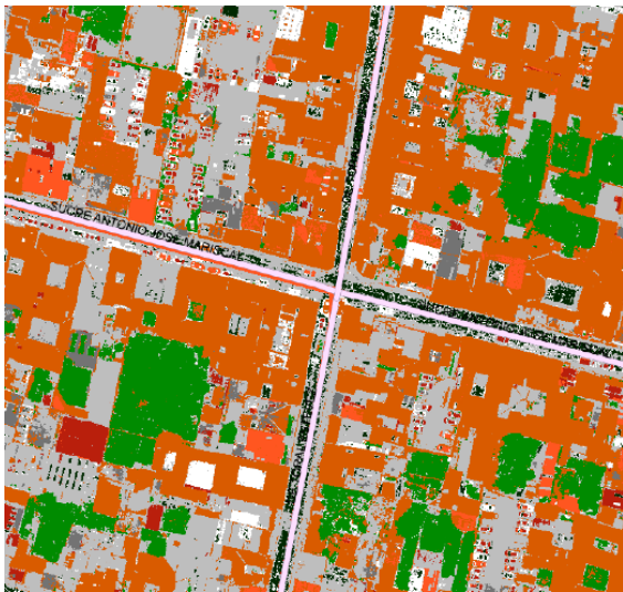
Figure 4. (b) 2016 raster image, 2,5cm/px. This image was classified and generalized with the SVM lineal function. Source: Authors, 2016
