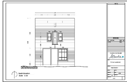
Figure 9: Examples of architectural plans created by Farzan Baradaran from the point cloud data. Source: Peter Dawson
