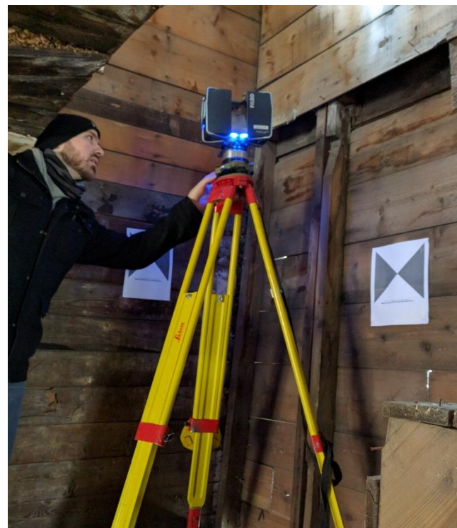
Figure 5: Scanning the interior of the laundry shop using the Faro Focus 3D scanner. Source: Peter Dawson.
