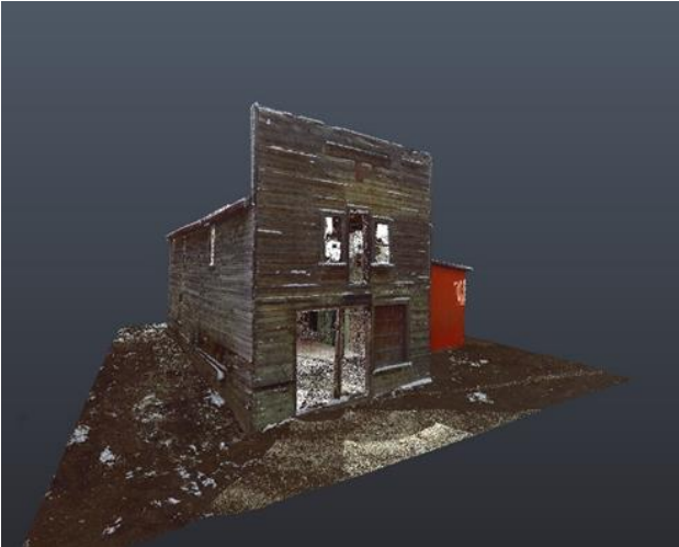
Figure 6: The registered point cloud for the complete building. Source: Peter Dawson
