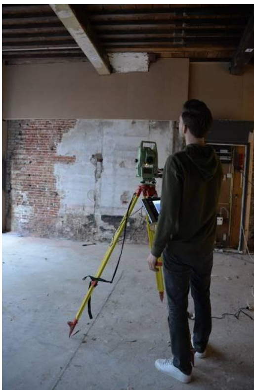
Figure 4. Recording targets with a Total Station connected to a tablet with BricsCAD to support the photogrammetric survey
