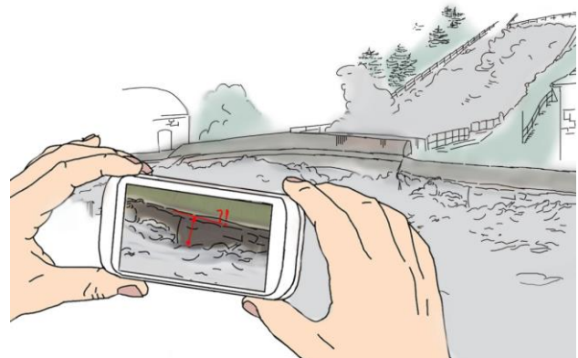
Figure 1. Schematic use case of water level determination using hand-held smartphone.
