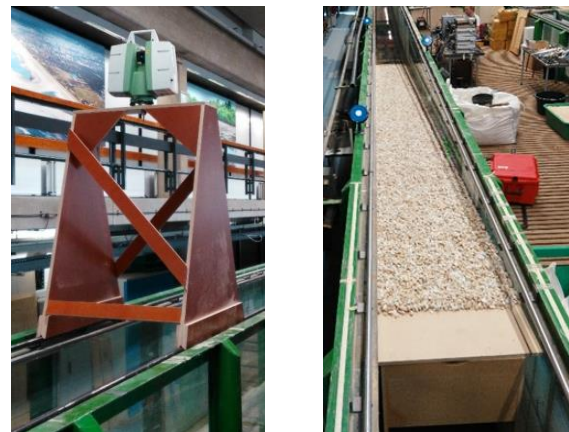
Figure 2. Left. Special wooden construction for mounting the laser scanner above the flume. Right. Scanner view of the scene. The along flume direction is denoted Y in this work, and the across flume direction X, in the local slope coordinate system.
