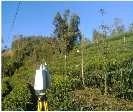
(a) Scanning tea plants on a slope by using the LiDAR.
