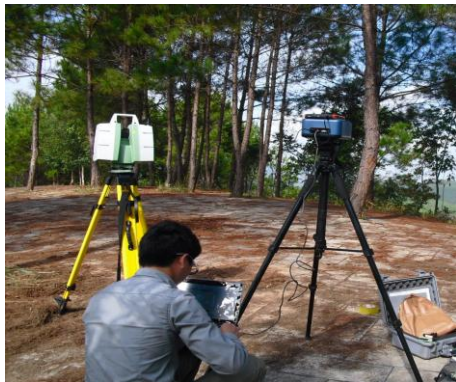
(b) Scanning coniferous trees by using the LiDAR and imaging spectrometer.
