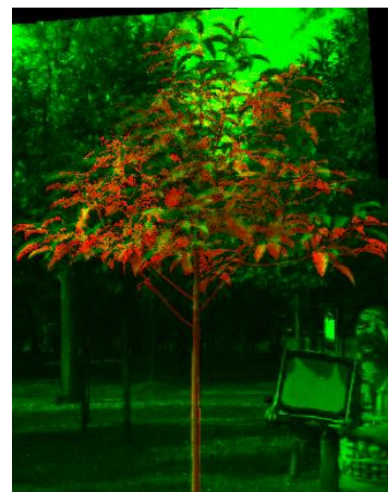
Figure 4. A Pseudo-color image of a pair of co-registered data. Here laser point cloud data is shown in red, and imaging data are given in green.
