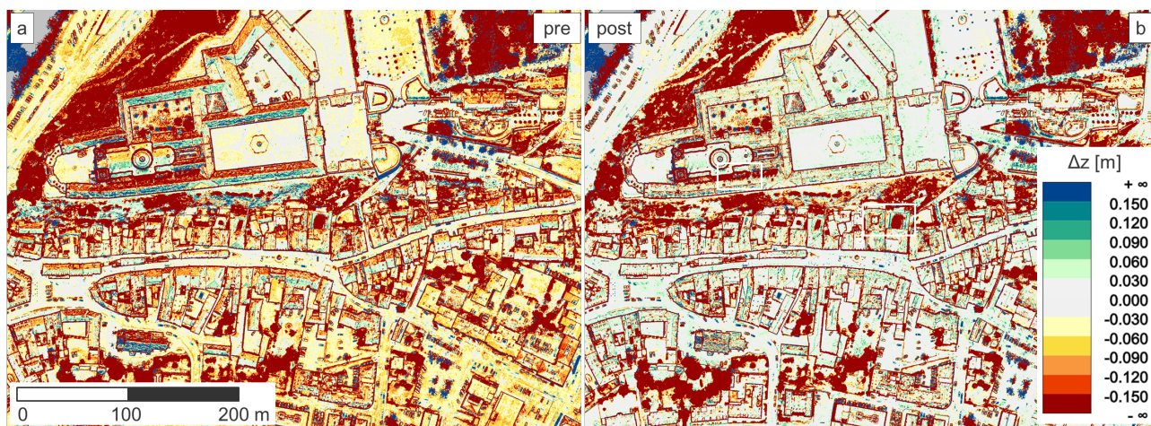
Figure 7. Color coded height differences LiDAR vs. DIM before (a) and after (b) simultaneous orientation of scans and images
