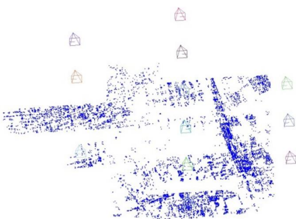
Figure 3. The reconstructed 3D features (blue points) and the camera centres (triangular cones)
