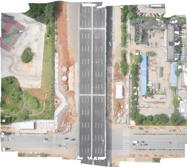
Figure 4. The ortho-rectification and mosaic result of the UAV dataset
