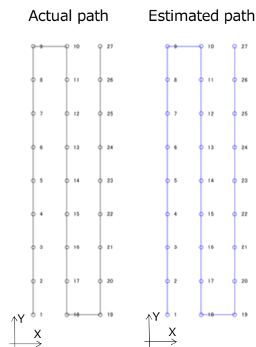
Figure 9. Camera translation estimation result, Elevator hall (Left image: actual camera path, right image: our estimated result)
