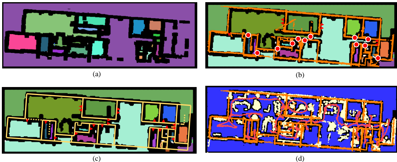
Figure 9. (a) Top view of space partitioning without using openings and wall information. Colored areas are empty spaces and black areas show the position of walls and clutter. (b) Space partitioning results after modification with openings and wall information. The overlaid orange layer show detected walls. Red dots show detected doors and red triangles show undetected doors. (c) Space partitioning and original floor plan. Light green area in the bottom of figure shows not correctly divided partitions. Small red triangles show the location of correct doors. (d) Navigable space (blue), clutter (yellow), and trajectory (coral).
